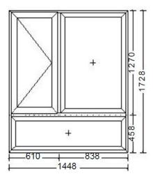
Pos: W2A Qty: 3 Area including Insertions: 2.1m<sup>2</sup> Frame: 1448x1448mm Sash: 914.5x939.5mm, 443.5x950.5mm, 1392x407.5mm
