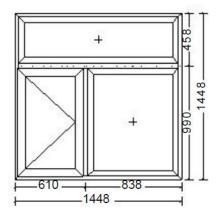
Pos: W1A Qty: 4 Area including Insertions: 2.5m<sup>2</sup> Frame: 1448x1728mm Sash: 1392x407.5mm, 570.5x1230.5mm, 787.5x1219.5mm
