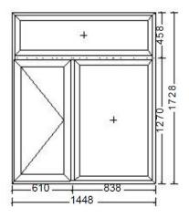
Pos: W2 Qty: 48 Area including Insertions: 2.1m² Frame: 1448x1448mm Sash: 570.5x950.5mm, 787.5x939.5mm, 1392x407.5mm
