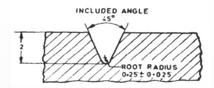
Fig. Enlarged view of notch for square test piece
