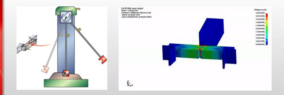
IS1757 / ISO148-METALLIC MATERIALS — CHARPY PENDULUM IMPACT TEST
