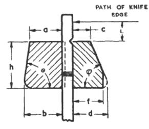
Note  $\leftarrow$  Dimensions a, b, c, d, e, f, g, k, and the angle  $\theta$  and should be obtained from the actual grips in the machine, the dimension h should be checked and, if necessary, corrected to make L equal to 22 mm.
