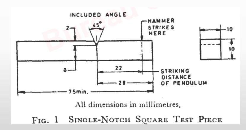
IS 1598 **METHOD** FOR IZOD IMPACT **TEST OF METALS**
