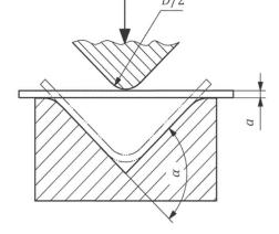
Figure 2 — Bending device with a V-block and a former
