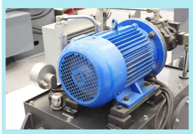
**SCOPE**- IS 12615 covers the efficiency classes and performance specifications of single-speed line operated a.c. motors that are rated for operation on a sinusoidal voltage supply and : a) Have a rated power from 0.12 kW to 1 000 kW; b) Have 2, 4, 6 or 8 poles; c) Have a rated voltage Un up to 1 000 V with a rated frequency of 50 Hz.
