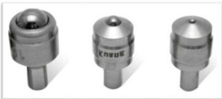
Fig. Real Life Images of Brinell Hardness indenter
