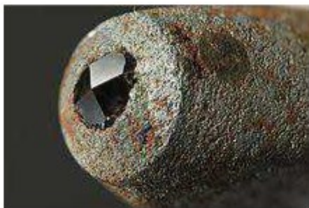
Fig. Real Life Image of Vickers Hardness Indenter
