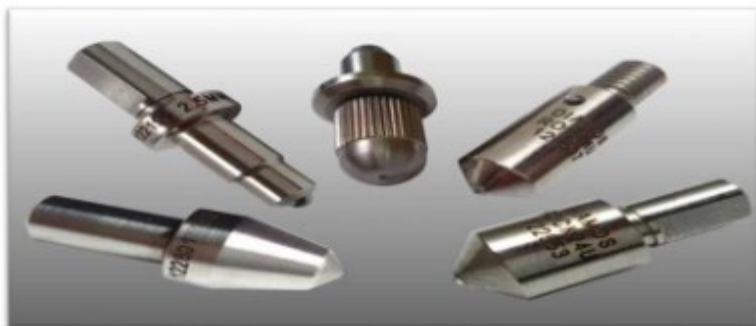
Fig. Real Life images of Rockwell indenter
