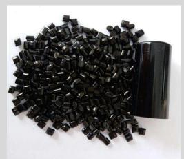
Carbon black absorbs light from the entire range of the solar spectrum and protects the interior of the plastic from the penetration of high energy photons thereby protecting the chemical cross-linking and bonds. Stability of tank is very important when the material is subjected to exposure to sunlight and weathering over long periods of time. Hence most of the HDPE Tanks are black in colour for increasing the life.
