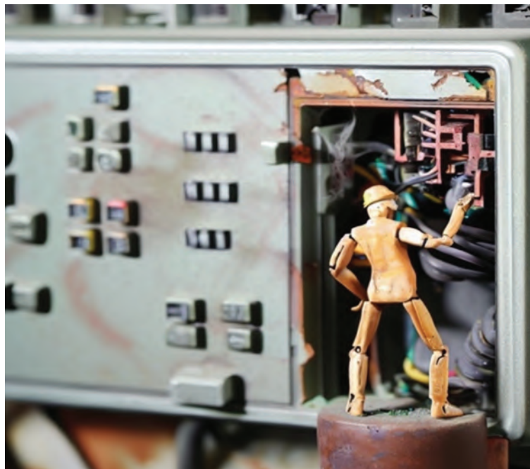
Figure 3 Damaged electric panel can be a potential hazard in a machine tool
