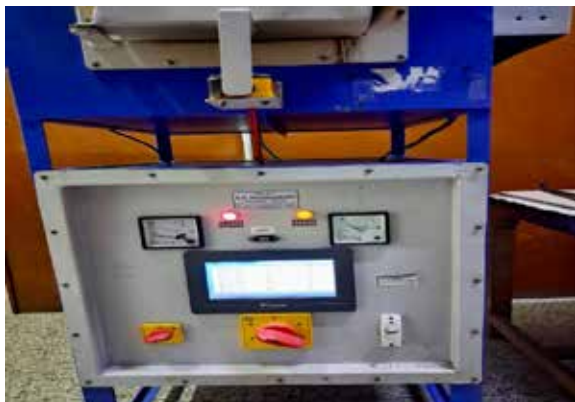
Muffle Furnace equipped with Data logging facility
