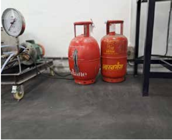
LPG Cylinder which have undergone Burst Test
